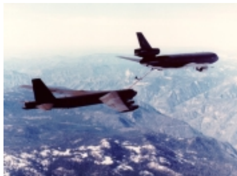
KC-10 and B-52. Air refueling increases an aircraft's range and is crucial for global attack missions.
